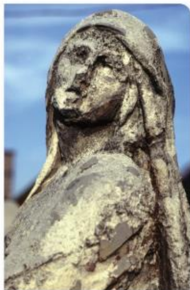
Fig. 25.32 The effects of acid rain on a statue
