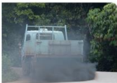
Fig. 25.31 Vehicles with poor maintenance release black smoke
