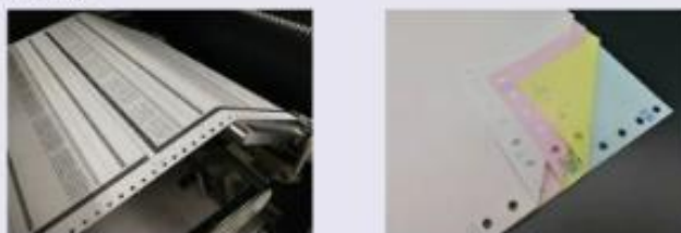
Fig. 1.49 Dot matrix printer (left) and multipart forms (right)
