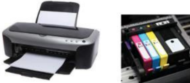
Fig. 1.47 Inkjet printer (left) and ink cartridge (right)
