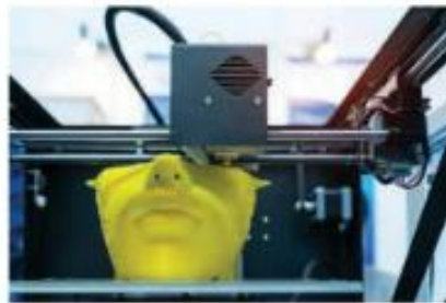
Fig. 1.51 3D printer printing a mask
